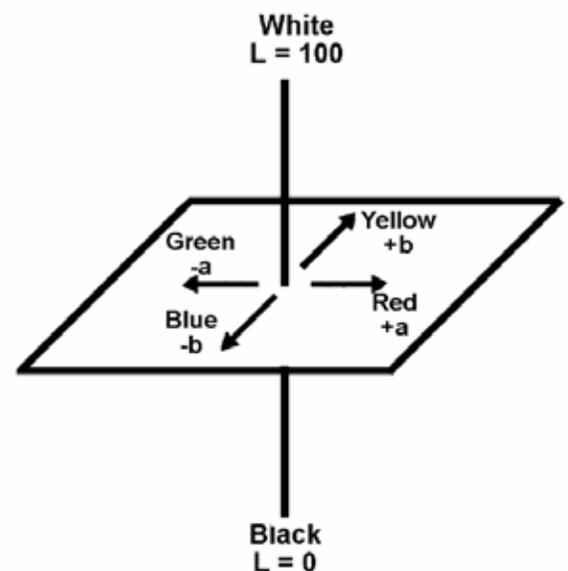
The Hunter L, a, b color space is organized in a cube form. The L axis runs from top to bottom. The maximum for L is 100, which would be a perfect reflecting diffuser. The minimum for L would be zero, which would be black. The a and b axes have no specific numerical limits. Positive a is red. Negative a is green. Positive b is yellow. Negative b is blue.
